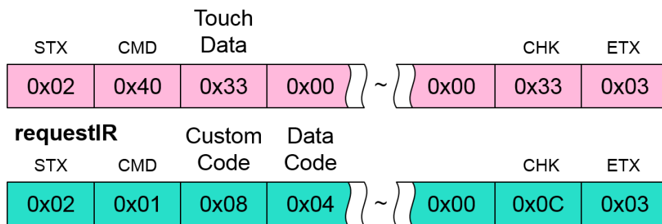
Figure 2-4 Example of transferring custom code 0x08 and data code 0x04
